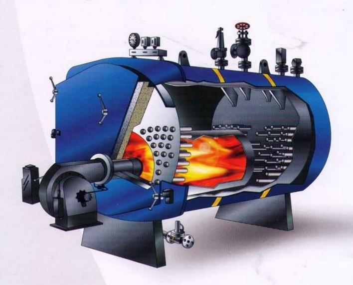
THE TITAN PACKAGE STEAM BOILER MODEL 'AS' IS DESIGNED TO THE LATEST BRITISH STANDARD 2790. THE BOILER ADOPTS THE REVERSE-FLAME PRINCIPLE OF COMBUSTION WHERE THE HOT GASES MAKE 2 PASSES WITHIN THE PRESSURISED COMBUSTION CHAMBER AND THE THIRD AND FINAL PASS THROUGH THE FIRE TUBES ON ITS EXIT TO THE CHIMNEY.
